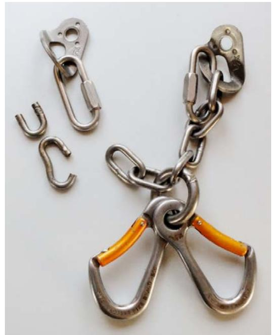
Photo 1: The FIXED-balancing anchor in which two chain links are broken.
