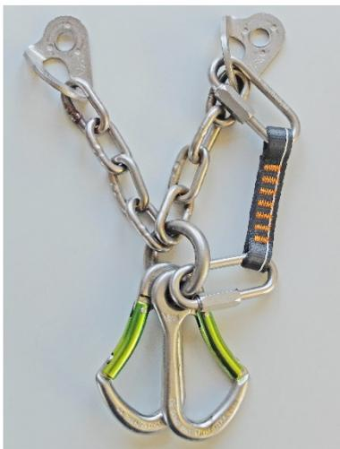
Photo 2: Example of a temporary makeshift rear backup.
